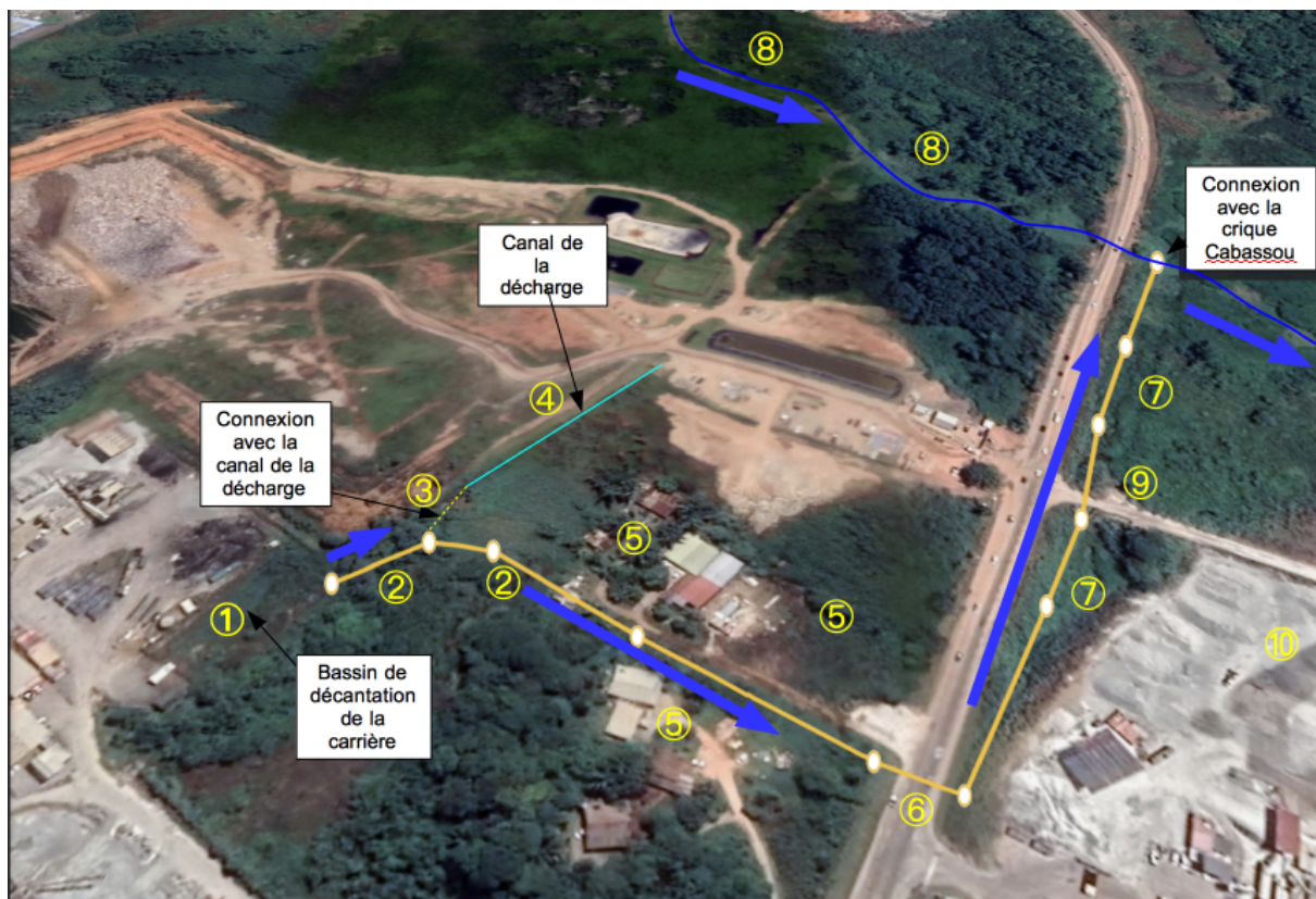
Figure 24 : Circuit hydraulique initial probable (source Google Earth)
